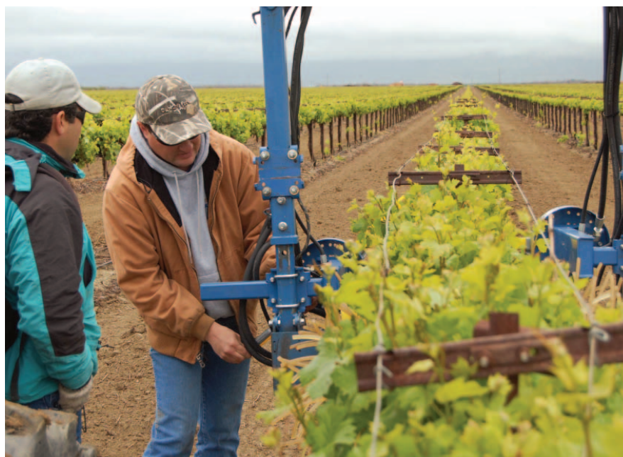
Adjustments were made in the vineyard to the shoot thinning equipment to improve performance. Photo: S. Kaan Kurtural, Fresno State
