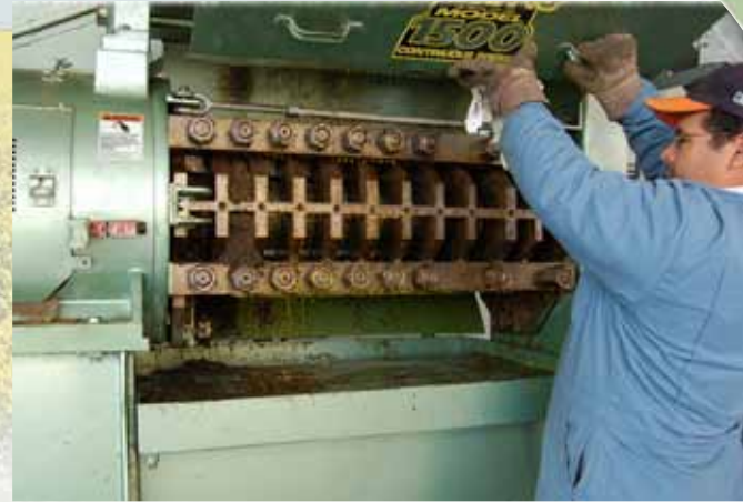
Mechanic Jose Lopez adjusts horizontal oil press during canola and mustard seed processing at Red Rock Ranch.
