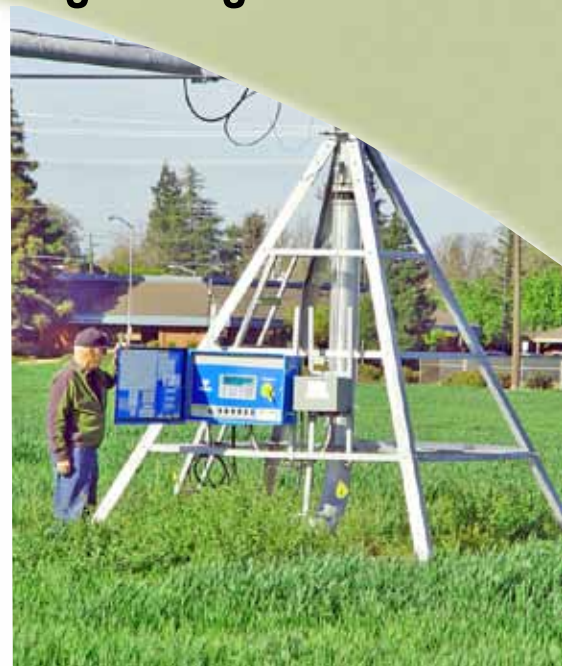
CIT agricultural engineer Ed Norum monitors control panel for new center pivot irrigation system at Fresno State's University Farm.
