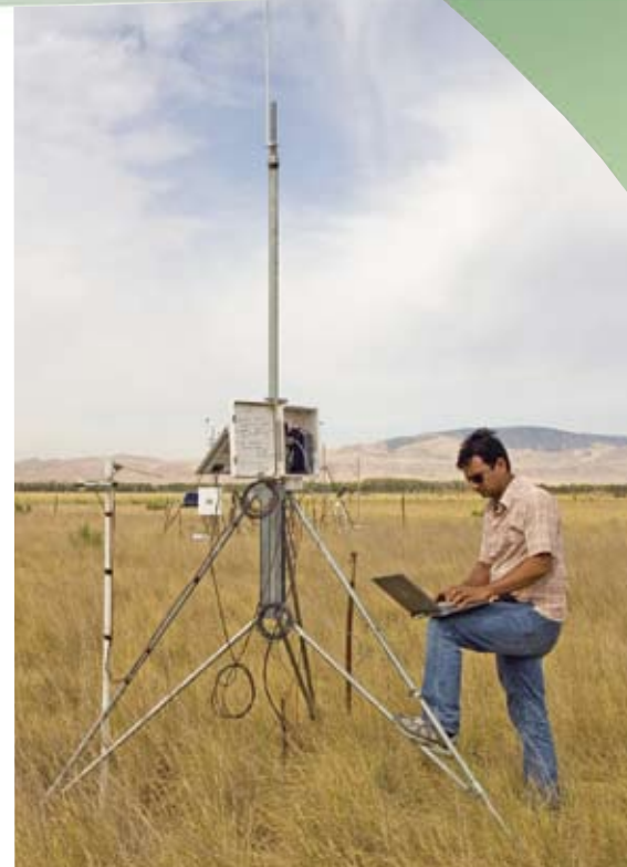
CIT irrigation scientist Diganta Adhikari monitors information collected by a surface renewal weather station during West Side experiments.
