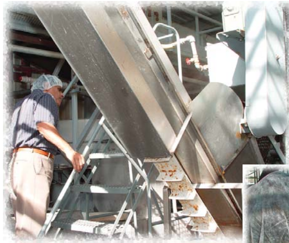
Fresno State food science professor Gour Choudhury examines the output conveyor of the prototype lye-peeling unit. The unit operates at approximately one-fifth the capacity of a standard commercial peeler.
