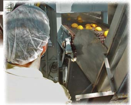
Fresno State food science professor Gour Choudhury examines the output conveyor of the prototype lye-peeling unit. The unit operates at approximately one-fifth the capacity of a standard commercial peeler.
