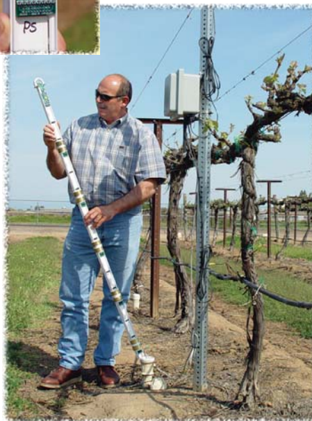
Right: Matt Angell, vice president of sales for PureSense, displays a five-foot-long soil moisture sensor pulled from its underground sleeve. Above: Close-up of on-board computer at top end of sensor.
