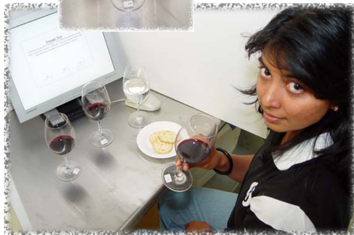
Master's degree enology student Amita Shingre demonstrates a typical triangle test of wines in the Sensory Laboratory at Fresno State's Viticulture and Enology Research Center.
