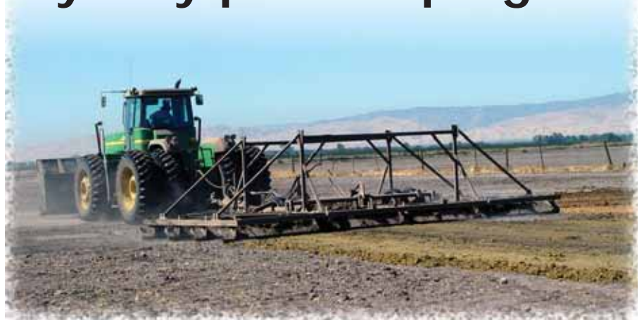
A tractor with grader spreads food processing by-product residues onto a field for use as a soil amendment. The residue will be allowed to dry, then disked into the soil.
