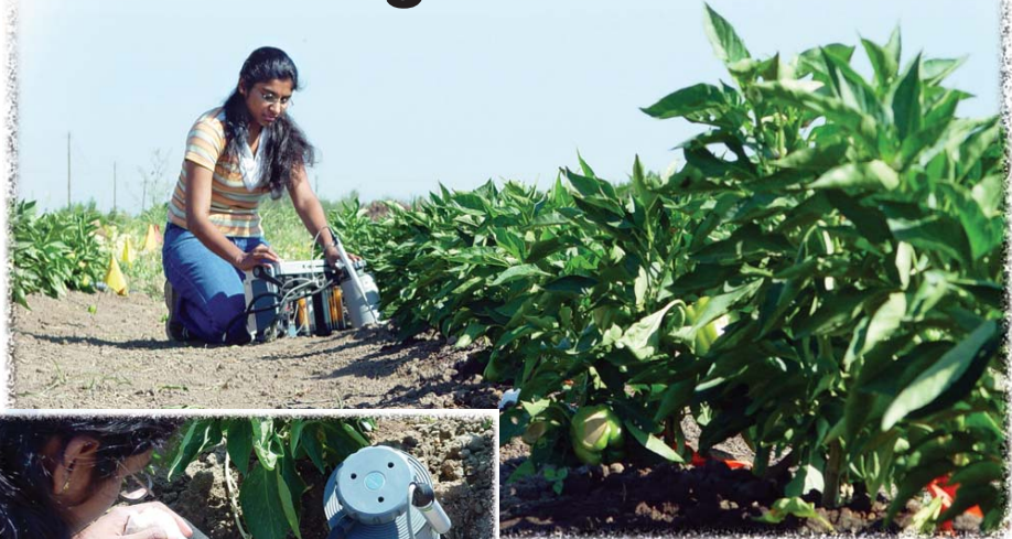
Above: Graduate student research technician Namratha Reddy tracks soil moisture conditions in an experimental plot of Bell peppers being grown organically with the AirJection® system.
