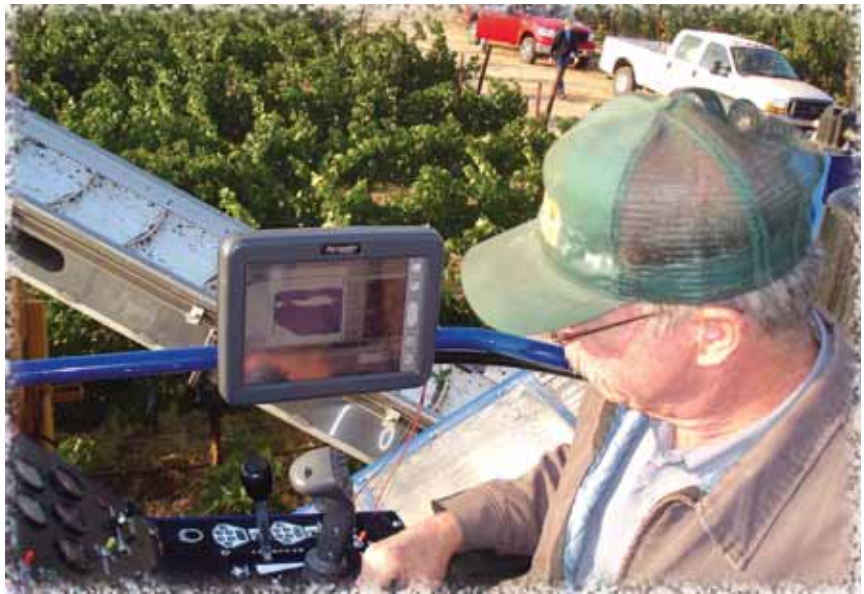
Harvester operator Mike Fitzgerald of Oxbo/Korvan Inc. assesses control information from a computer monitor perched at eye level along the harvester’s top railing. The monitor displays images showing what sections of the field are being harvested.
