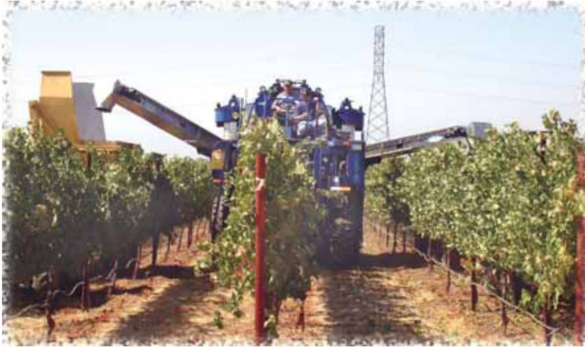
A mechanical grape harvester guided by computerized geographic information systems (GIS) technology picks grapes during an experimental harvest last September.
