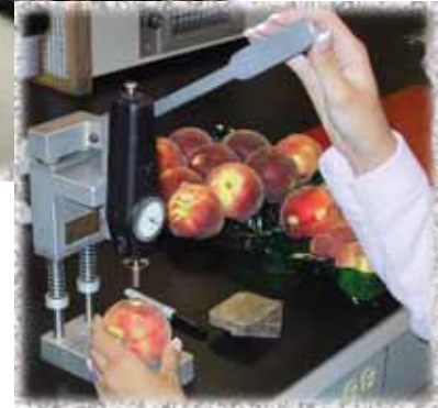
Below: Peach fruit flesh firmness is measured using a penetrometer
