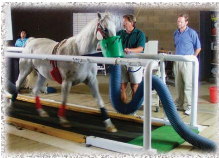
Specially designed equine treadmill enables Cal Poly Pomona professor Steven Wickler (left) to measure the metabolic effects of walking and trotting.
