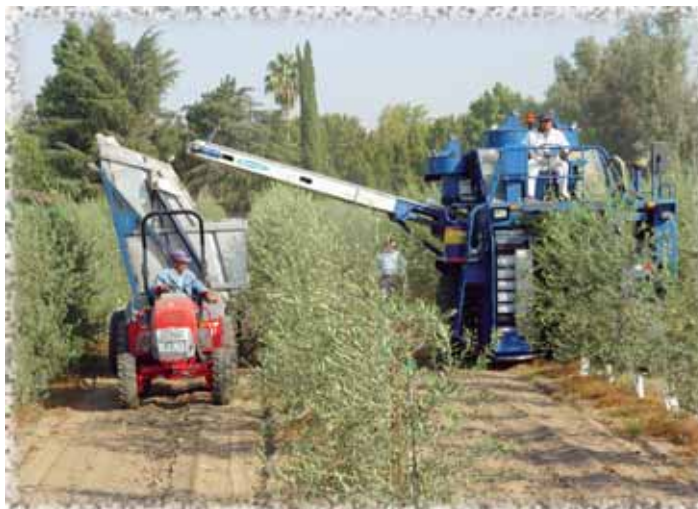
Left: A converted grape harvester machine picks olives on a 20-acre experimental plot on Fresno State's university farm
