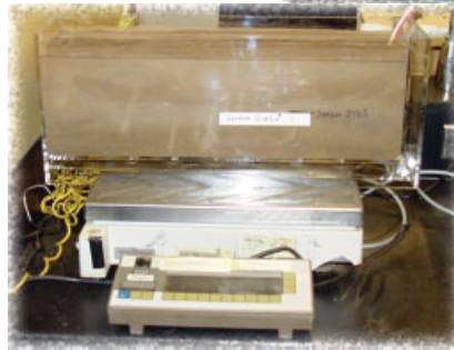
Above: Research analyst Diganta Adhikari downloads moisture data from sensors embedded in a soil sample. Left: Initial soil moisture content is determined by weighing sample.
