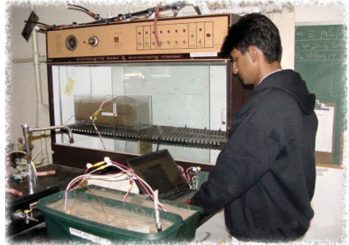
Above: Research analyst Diganta Adhikari downloads moisture data from sensors embedded in a soil sample. Left: Initial soil moisture content is determined by weighing sample.
