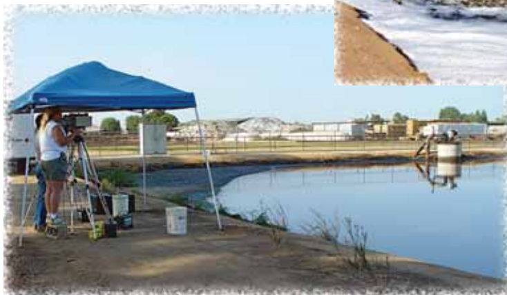
Above: Typical dairy lagoon aeration process. Left: Fresno State researchers use tunable diode lasers to measure ammonia and other gas emissions above lagoon.
