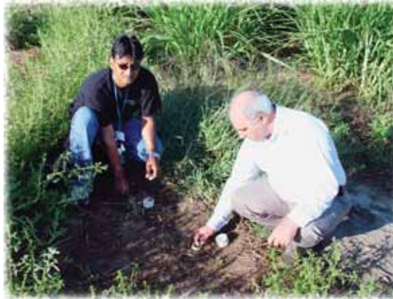
CIT research technician Diganta Adhikari (left) and Mohammad Moaddab, reclamation coordinator for the Fresno wastewater treatment plant, check lysimeters used to collect soil water samples.
