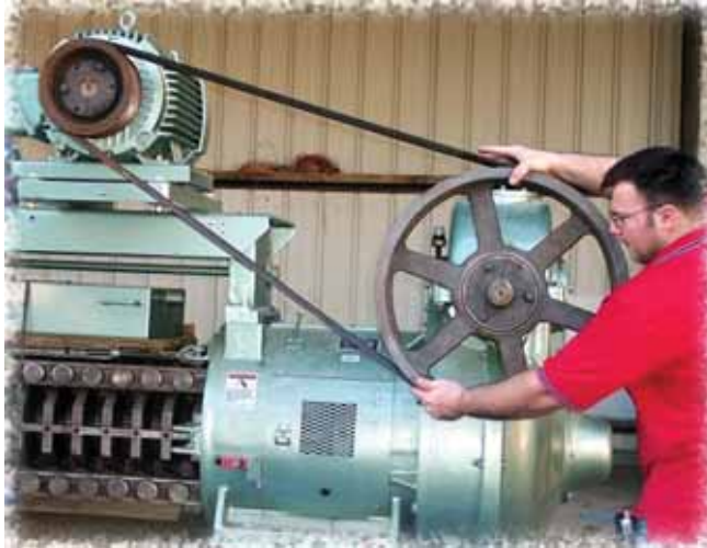
Fresno State student research technician Justin Ferreria examines pulley belt on a newly-installed press that will be used to extrude canola oil.
