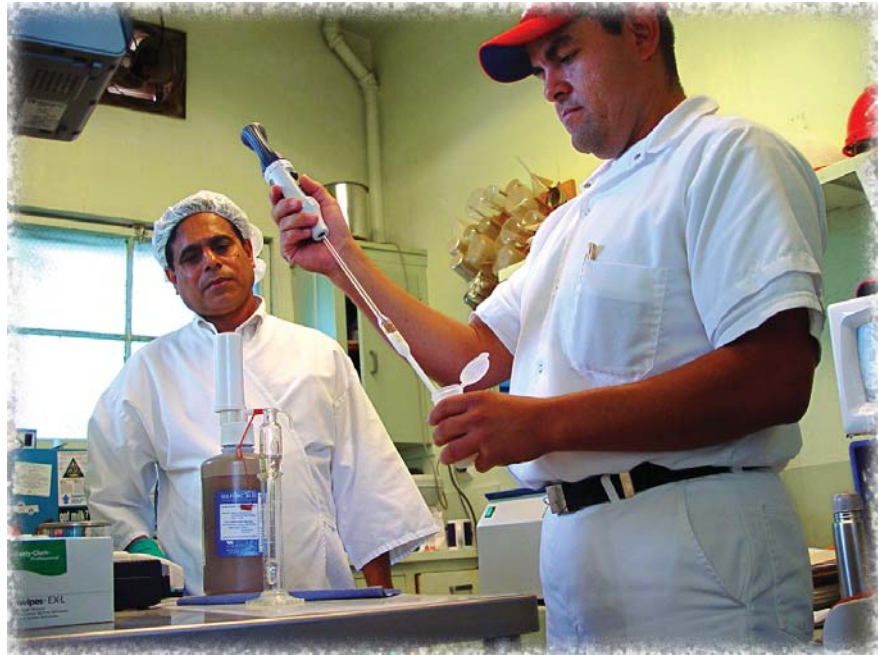
Gour Choudhury (left) watches as Daniel Avila, head technician for Fresno State's dairy products processing unit, tests the acidity level of milk in the laboratory.
