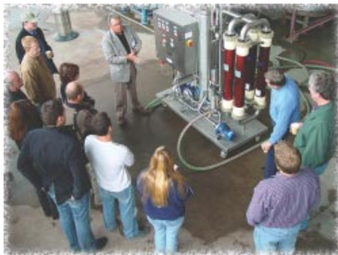
Pall Corp. wine system sales manager Allen Posella demonstrates a crossflow filtration unit to students and wine industry members during a workshop held at VERC.
