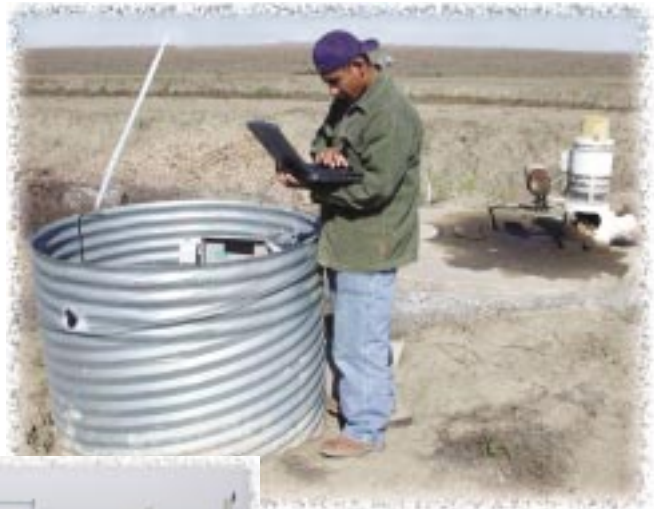
Top photo: Student research assistant Xavier Arellano uses a laptop computer to download drainage flow data in the field. Left: A row of 36 column lysimeters enables researchers to test salt tolerance of various crops.
