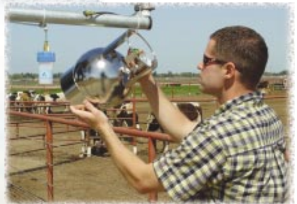
At left, tower unit with air sampling equipment stands downwind of San Joaquin Valley dairy. Above, student research technician Matt Beene adjusts flow level of vacuum canister used to collect air samples.
