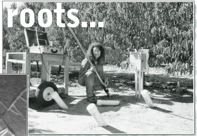
Fresno state graduate student Elizabeth Dickson kneels by the underground tubes through which a video camera takes images of peach tree roots using a minirhizotron camera system. Photo at left shows sample picture captured by the camera.
