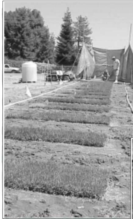
Field researcher Cindy Garretson (kneeling) of the Department of Pesticide Regulation prepares a turf plot for sprinkling during tests measuring diazinon runoff. Assisting in project operations (right) is CIT research technician Hercules Gonsalves. Bottom photo: One-liter bottles collect runoff water at end of each turf plot.
