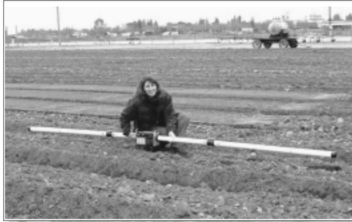
New CIT research scientist Florence Cassel Sharmasarkar holds an electronic device for measuring electromagnetic inductance (EM) in the soil. Data will be used to help determine moisture content.
