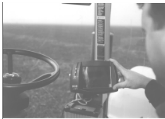
Custom equipment operator Patrick Boyle of Fresno shows the GPS computer programming screen inside the tractor cab.
