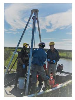
Figure 7.—Cooper Nichols, Jerome Langlinais, and Aaron Friend (left to right) extract a core sample along the shoreline of the marsh. Image at right the core sample exposed.
