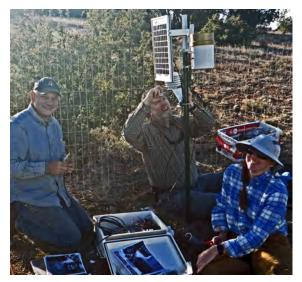
Figure 2.—Harry Hosler (left), Greg Anderson, and Amber Riordan (right), from the Flagstaff and Globe Soil Survey Offices work to install the Disterheff soil climate station.
