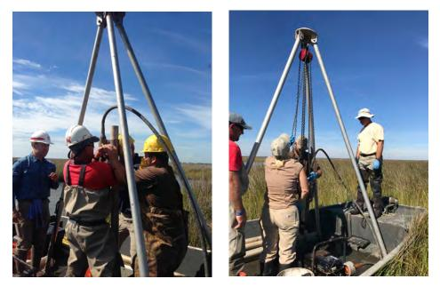
Figure 8.—Left: Jerome Langlinais observes while Rob Tunstead, Aaron Friend, and Cooper Nichols insert the aluminum tube attached to vibracore. Right: Alison Steglich hoists the tube using block and tackle mounted to a tripod.
